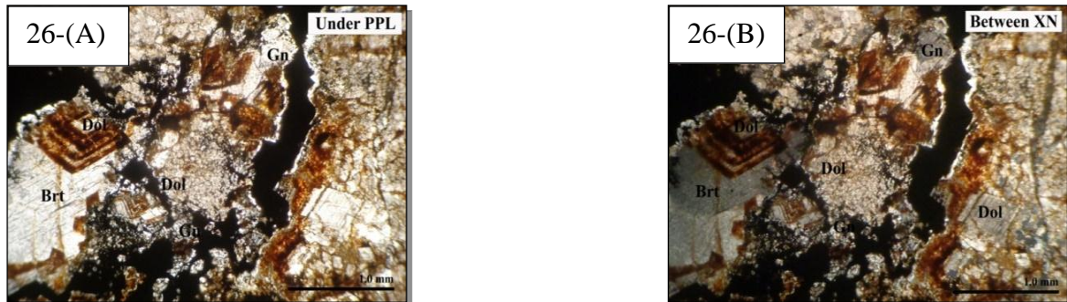
Figure 26 Thin section Photomicrographs showing dolomitization with Pb mineralization Under PPL & Between XN (Dol= Dolomite, Gn= Galena, Brt=Barite)
